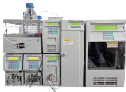
HPLC with High-pressure 6-way Switching Valve-UVD
