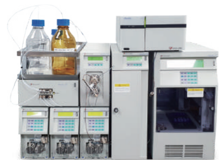
HPLC with High-pressure 6-way Switching Valve-PDA
